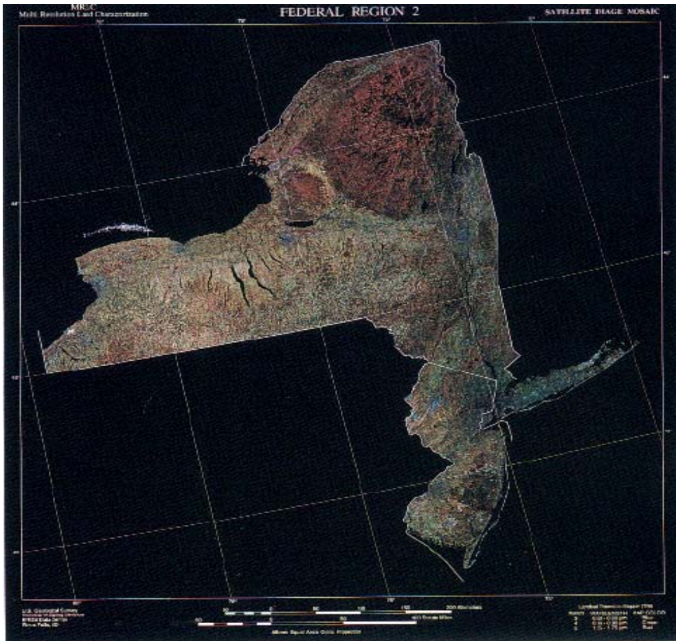
Fig. 1. Landsat thematic mapper mosaic of Federal Region 2 produced using bands 5, 4, and 3 in the order of red, green and blue. Data represent leaf-off conditions.
