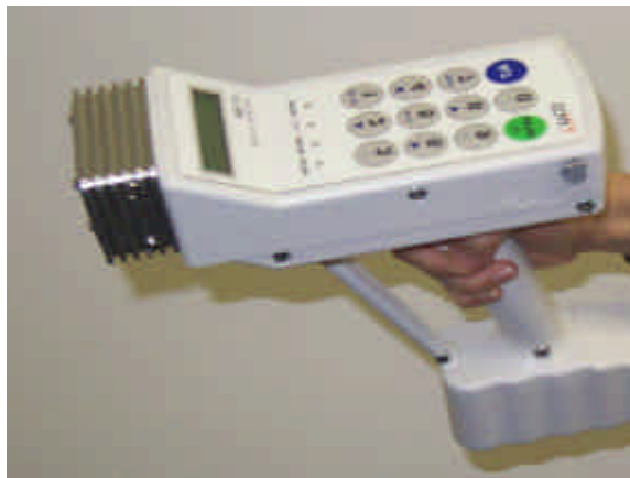
Figure 1. KeyMaster Technologies Pb-Test instrument.
