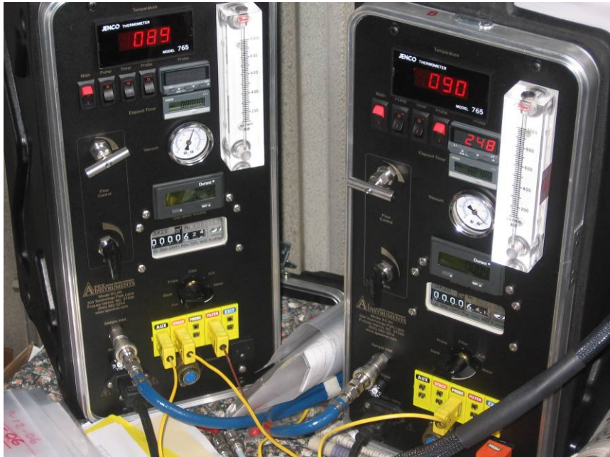
Figure 2-1. Apex XC-60 Gas Sampling Consoles
