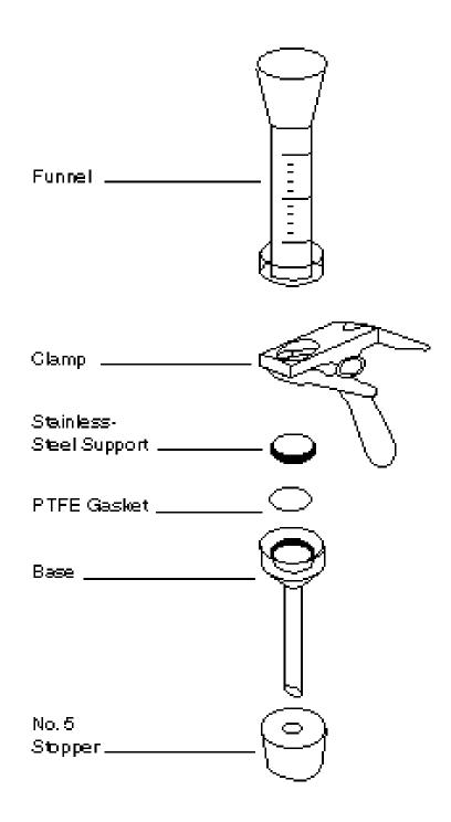
Figure 2. Filter Apparatus
