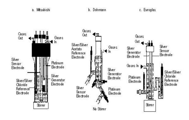
Figure 1. Microcoulometric Titration Cells (from Reference 7)
