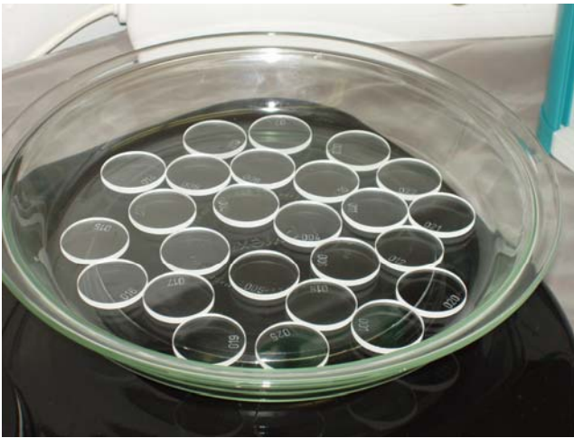
Figure 6-2. Quartz disks drying on a hot plate.
