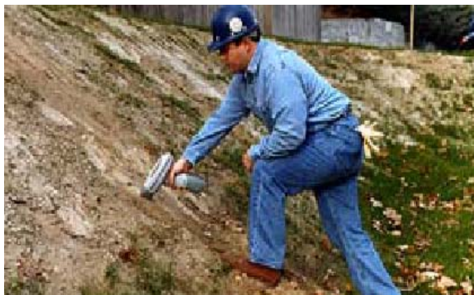
Figure 6-1. In situ testing with the Niton XLt 700 Series analyzer.
