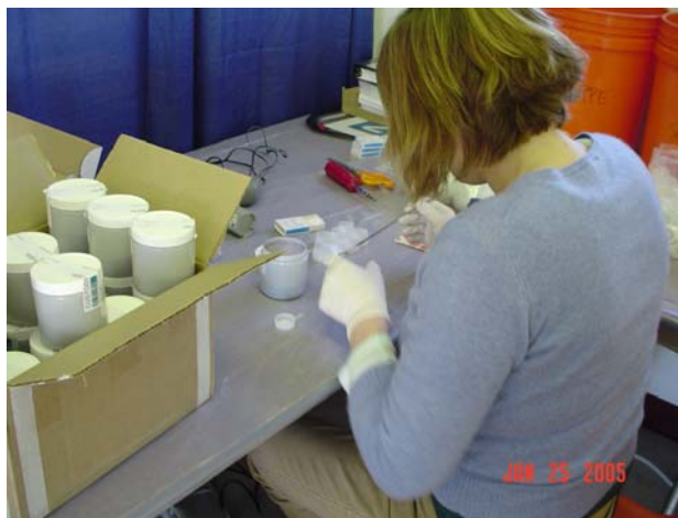
Figure 6-2. Niton technician using a stainless steel scoop to fill a sample cup.
