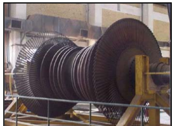
A power plant turbine rotor in line to be rebuilt.
