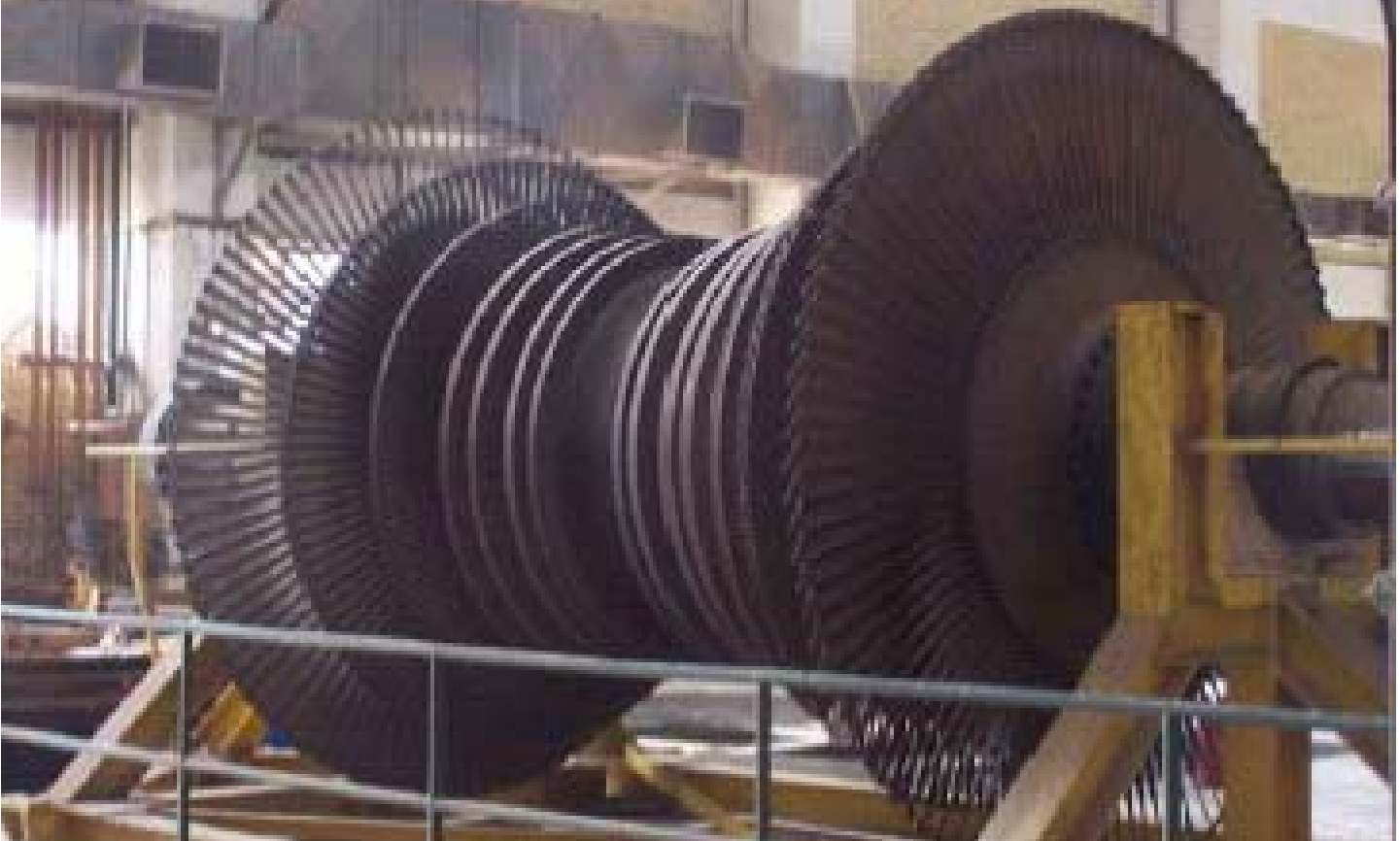
Above: A power plant turbine rotor in line to be rebuilt.
