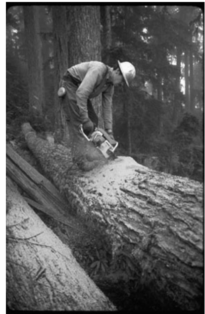
Sawyer cutting log to length for hauling to log deck - Salem District, OR.
