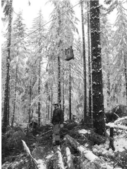
Logging using overhead cables during winter reduces impacts to soil and vegetation.
