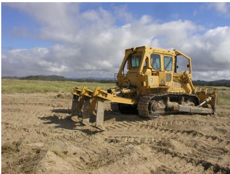
A Challenge Cost Share project to restore nesting habitat for the Western Snowy Plover, a species listed as threatened under the Endangered Species Act. The dozer is using a ripper attachment remove exotic, invasive European beach grass from 170 acres of a Habitat Restoration Area on the North Spit of Coos Bay, a BLM-managed area on the Oregon Coast.
