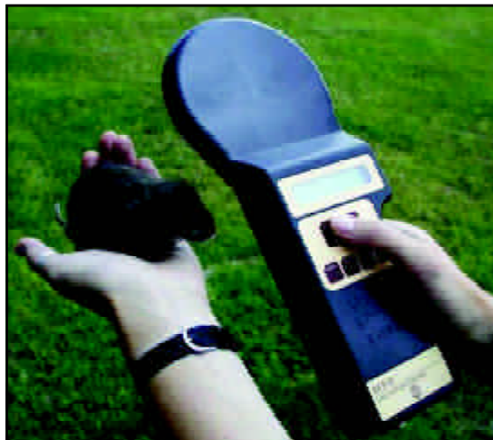
An electronic scanner reads the unique code from the microchip tag that has been inserted under the vole's skin.
