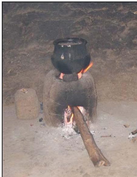
Figure 10: 6-brick stove plastered and installed in an IDP kitchen
