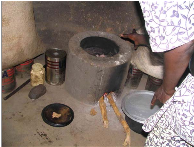
Figure 8: Molded 1-pot mud stove, promoted by NGO C in Gulu and Kitgum
