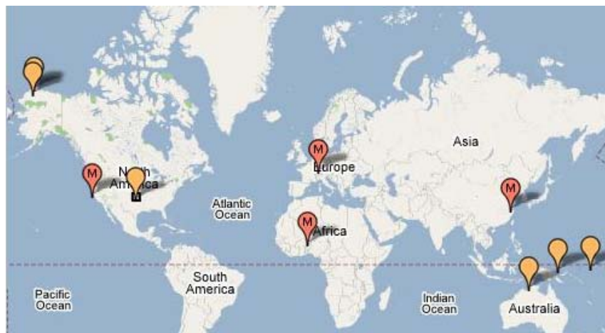
Figure 1: ARM Climate Research Facility measurement locations. Gold markers represent fixed-site locations in the North Slope of Alaska, Southern Great Plains of the United States, and Tropical Western Pacific. Red markers with “M” denote past (California; Niger), present (Germany) and future (China) mobile facility deployments.
