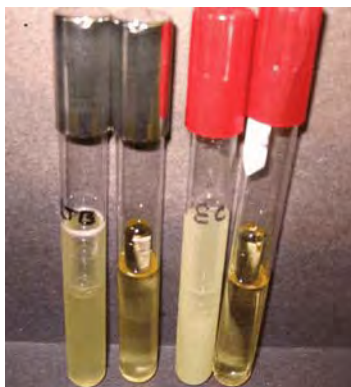
Photo 1. In LTB (two tubes on left with silver caps) and EC (two tubes on right with red caps), fecal coliforms produce turbidity and gas (tubes 1 and 3, when counting from the left).
