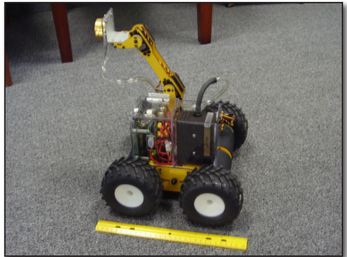
The PIPER is less than a foot long and a foot tall. Air samples enter the device through an adjustable vent and travel through tubing into a storage chamber on the chassis. (Photo courtesy of Stuart Shalat and the Robert Wood Johnson Medical School at the University of Medicine and Dentistry of New Jersey)
