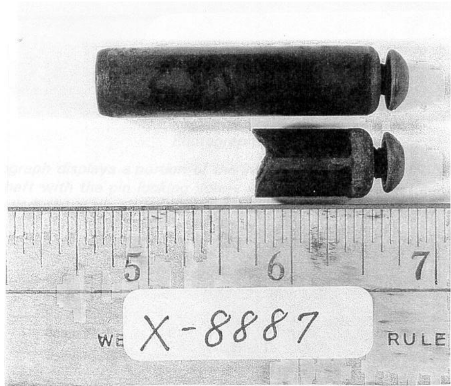
Figure E-15: Photograph shows the general configuration of the intact dowel pin removed from the idler shaft, and a portion of the fractured pin. Both pins exhibit the threaded machine screws, which were placed in holes drilled in the center of each pin to allow later pin removal.
