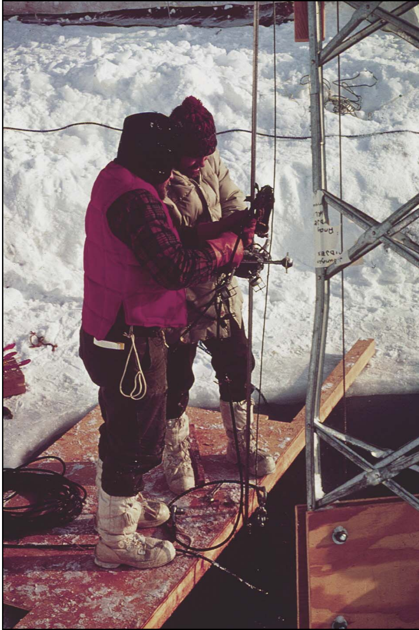
The author and Prof. J. D. Smith (red vest) deploying a Smith-rotor current meter triad in a large hydrohole during the AIDJEX 1972 Pilot Study north of Barrow, Alaska.
