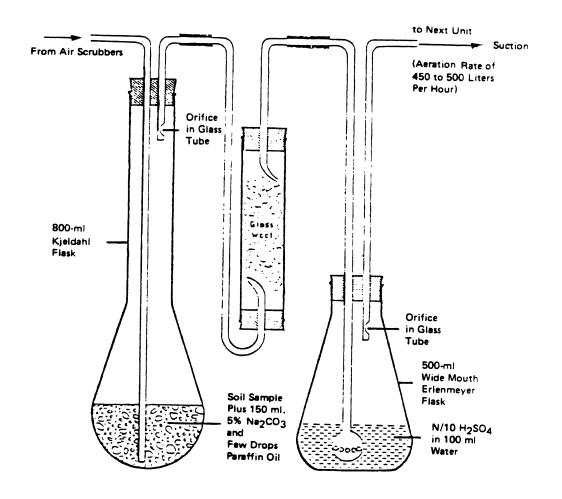
Figure 1. Diagram of aeration unit for determination of absorbed ammonia. Six to twelve such units is a convenient number for routine work; they can be mounted on a portable rack. (Apparatus as modified by Dr. A. P. Vanselow, Dept. of Soils & Plant Nutrition, Univerity of California, Riverside, Calif.).
