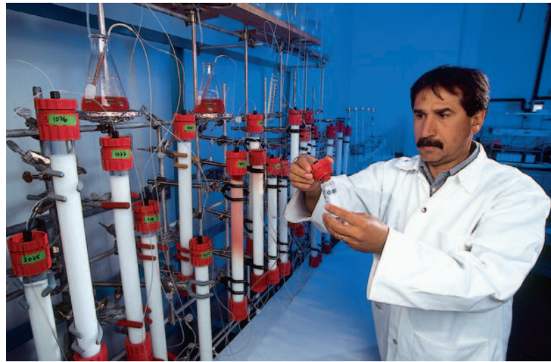
Mohammad Koohmaraie loads a muscle extract onto an ion-exchange chromatography column to isolate calpain and calpastatin.
