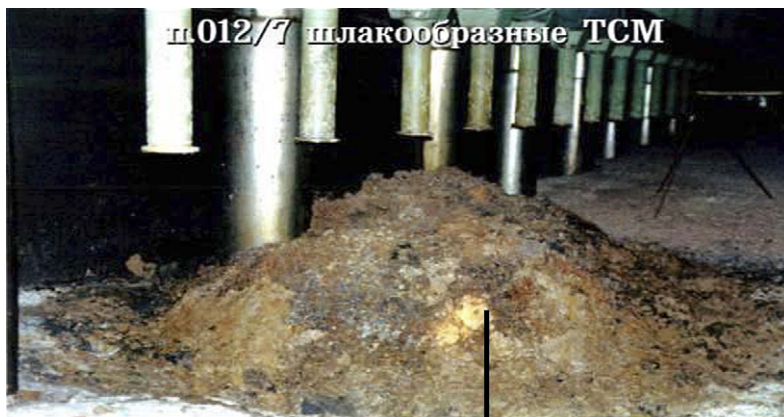
Fig. 8.10. “Chernobyl lava”, which primarily consists of the uranyl peroxide Studdite, a naturally occurring mineral that also forms from uranium decomposition in nuclear waste.
