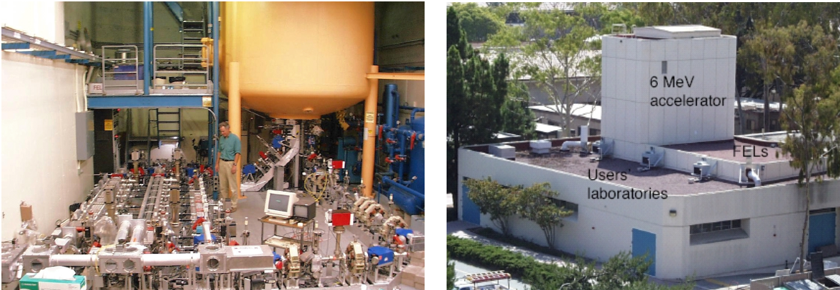
Figure 10.2 (left) Two free-electron lasers driven by a 6 MeV electrostatic accelerator in a ~1300 ft 2 vault. (right) The Center for Terahertz Science and Technology at UCSB.
