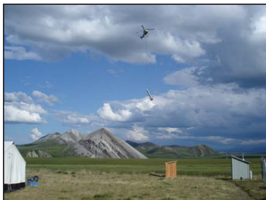
Airborne geophysical survey getting underway at the Ivotuk field camp in the southern National Petroleum Reserve–Alaska.
