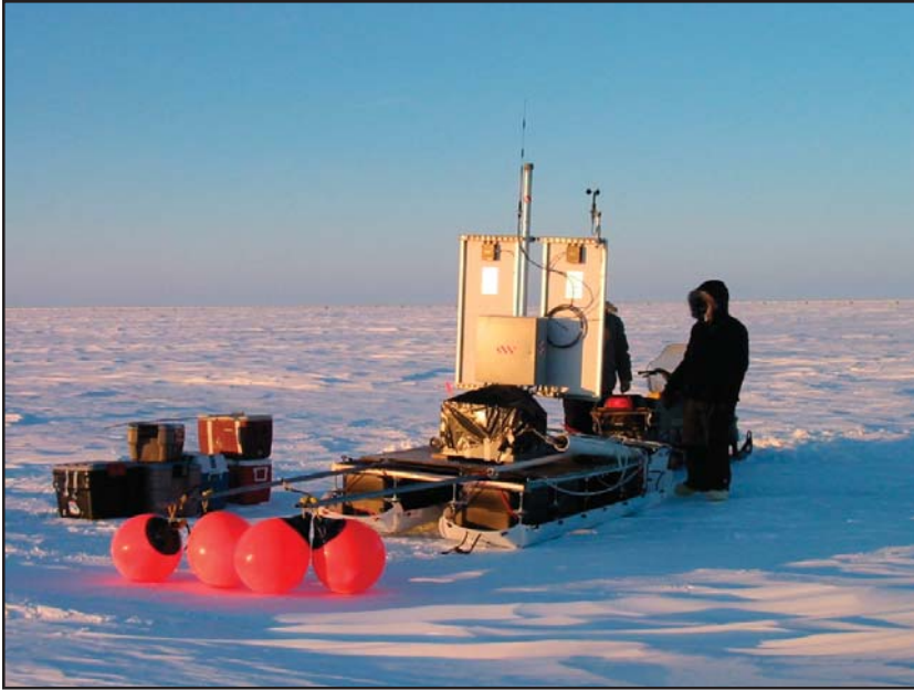
Transporting and setting up an instrumented raft for monitoring levels and chemistry of Arctic lakes.
