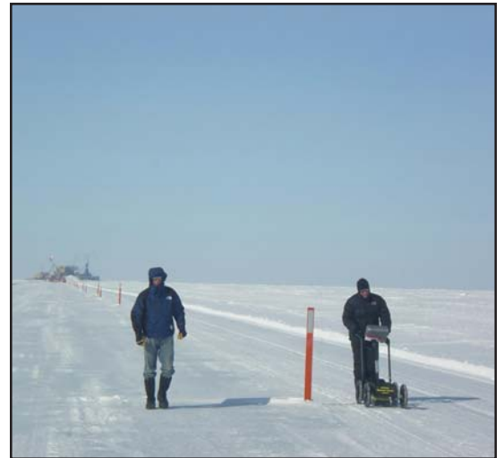
Radar team at Prudhoe Bay in April 2005 during cold weather reliability trials and thick ice (up to 6.5 feet) profiling without oil.
