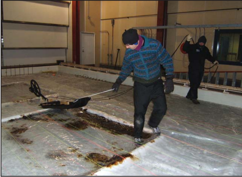
Radar team from Boise State University towing one of the two radar systems used at the U.S. Army Cold Regions Research and Engineering Laboratory to map oil under the ice in 2004.
