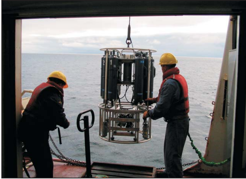
Researchers retrieving a CTD (conductivity, temperature, depth profiler) rosette on the USCGC Healy during the Shelf–Basin Interaction (SBI) study of the northern Bering Sea in 2005.
