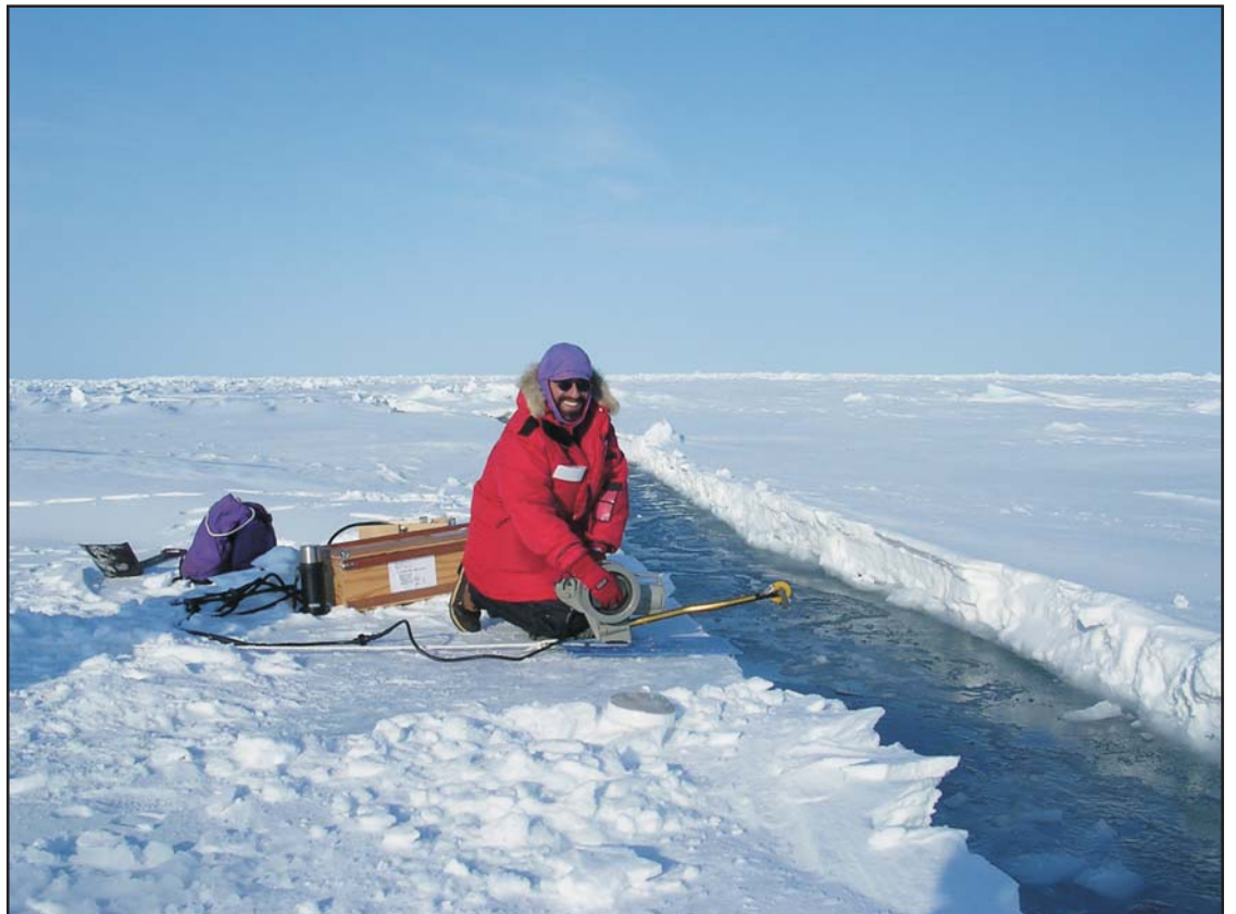
Scientist taking an ocean temperature and salinity profile at the side of a lead during field work.
