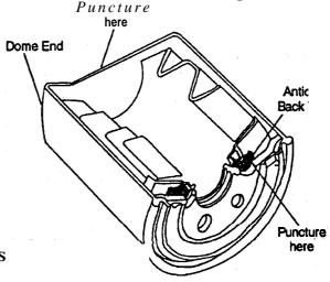
Turn the filter upside down in a used oil collection container, such as a drip pan. Drain as much oil as possible from' the filter. For best results, drain used oil filters for a minimum of 12 hours at an approximate temperature of 60F. (Oil filters also may be drained without puncturing them, and at cooler temperatures. The time required to effectively remove the used oil will take longer than 12 hours.)
