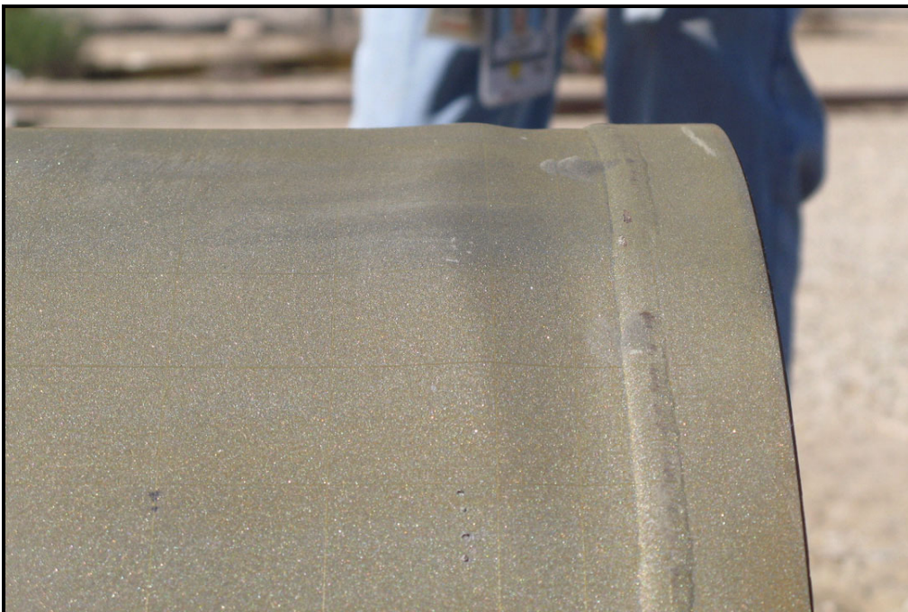
Figure 4-7 – SCA-1 Body Damage Side View, Bottom-Down End Drop Test
