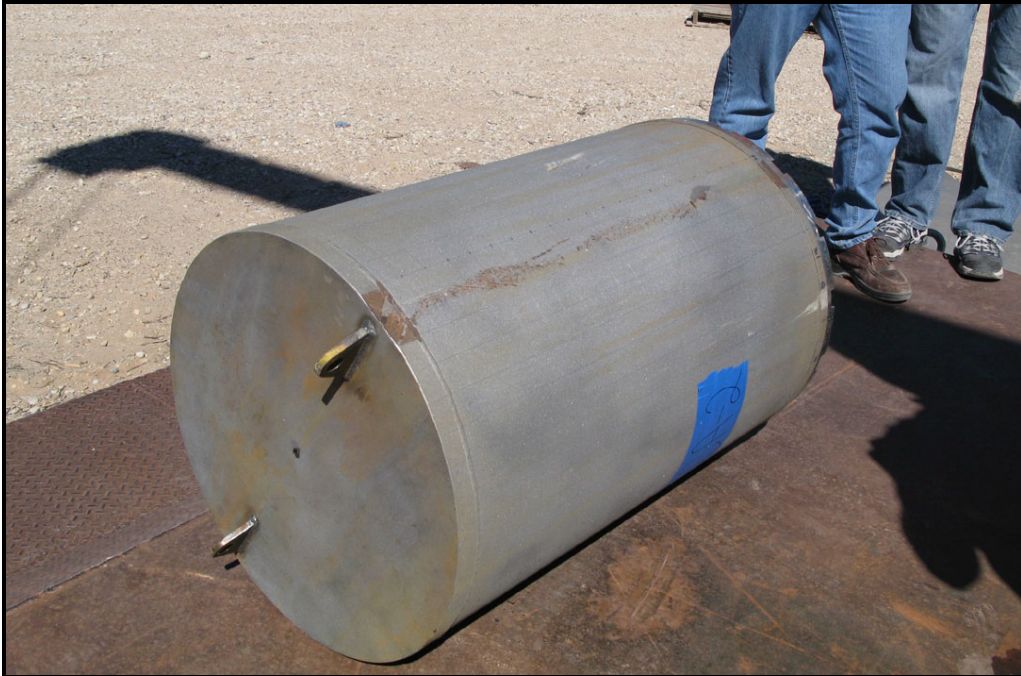
Figure 4-10 – SCA-2 Body Damage Overall, Side Drop Test
