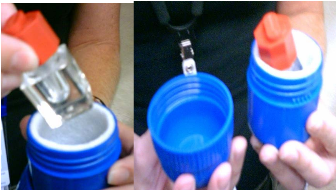
Figure 13. U.S. Department of Transportation (DOT) Type A Inner Containers
