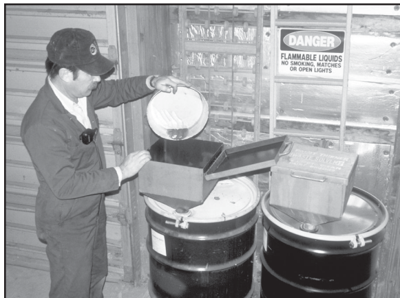
Figure 4-14. West Access Marina (Illinois) installed a high-temperature furnace in 1993, which extended the marina's boat maintenance activities into and through the winter. The marina's engine maintenance service collects between 1,000 and 2,000 gallons of waste oil a year. It is collected in small containers and stored in a 1,000-gallon drum. The furnace burns very cleanly at 3,000 EF. The furnace saves the marina thousands of dollars each year in waste oil removal costs (USEPA, 1996: Clean Marinas—Clear Value ).
