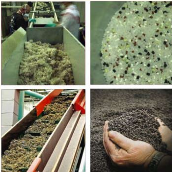
Conversion of reclaimed nylon (top left) and backing (bottom left) into new raw material feedstock (right)
