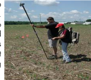
Figure 2. Measuring reflectance spectra of crop residues at BARC using a portable spectroradiometer and digital camera.
