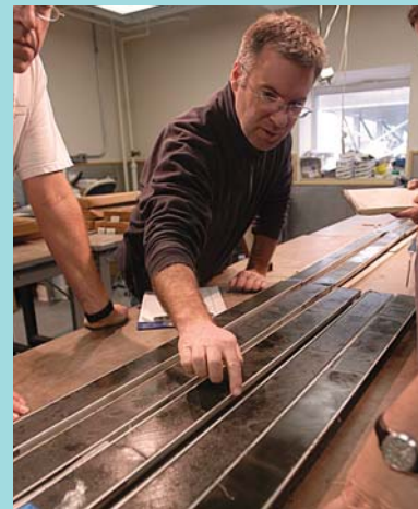
A scientist points to an interesting feature in a slide of sediment core as part of the Antarctic Geological Drilling program. Sediment and rock core were analyzed to study climate change. Credit: Peter West, National Science Foundation
