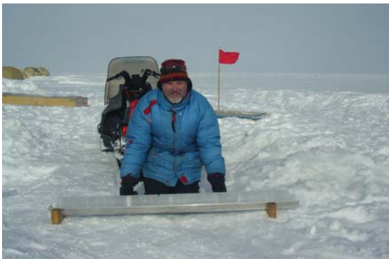
Bruce Vaughn displays a segment of ice core retrieved by the Center for Remote Sensing of Ice Sheets project. Note the narrow bands of white firn (layers of incompletely melted winter snow accumulation) between thick layers of translucent solid ice. Credit: Bruce Vaughn, Institute of Arctic and Alpine Research, University of Colorado
