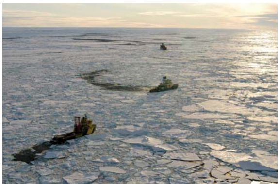
The Integrated Ocean Drilling Program completed the first-ever program of scientific drilling in the high Arctic with assistance from two icebreakers (background) that were used to protect the drillship (foreground). The results of the study are already revising our understanding of Arctic paleoclimate and the history of the Arctic Ocean basin. Credit: Martin Jakobsson © ECORD/IODP
