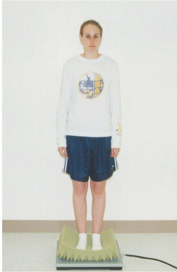
Figure 3.2. The experimental set-up used in the present experiment. Participants stood with feet together, arms by side, and looking straight ahead at a blank wall. A foam pad was placed on the force platform to create a compliant surface.
