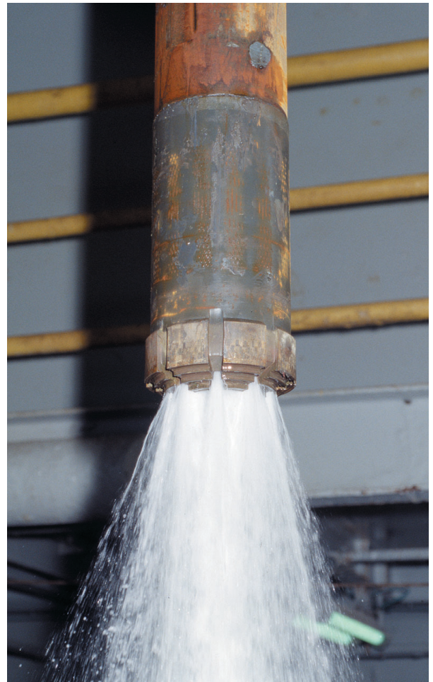
ADCB bit showing circulation test.
