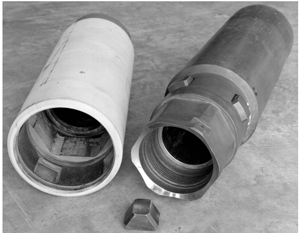
Photograph of the following MBR components: MBR Bit Disconnect, (left cylinder), Top Connector with hex drive (right cylinder), and Latch Segment (small pyramid-shape in the center).
