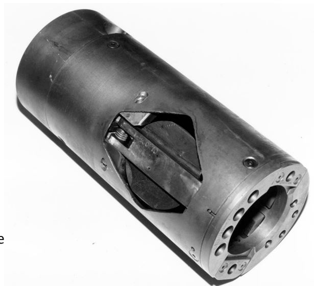
Photograph of the LFV showing the flapper in the locked-open position.
