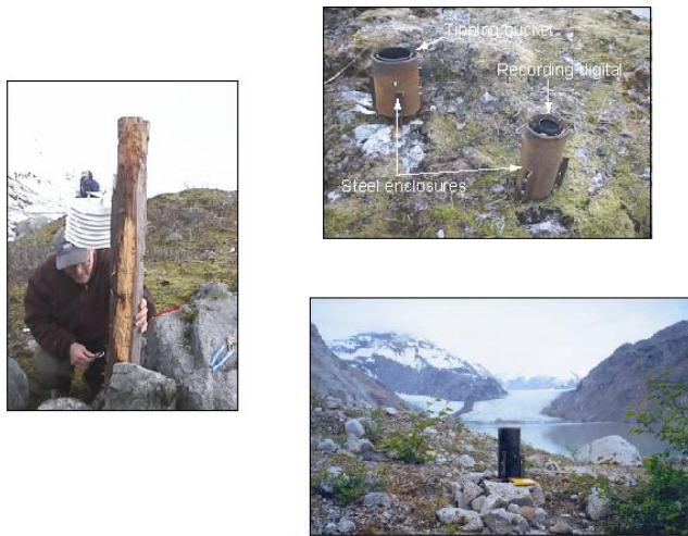
Figure 2. Typical rain and temperature gauge set up.
