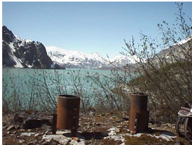
Figure 2. Typical climate sites. Upper left photo shows white solar radiation shield housing temperature sensors and a tipping bucket rain gauge installed on 1-meter tall post at Muir Glacier. Photo on lower right shows the tipping bucket and electronic rain gauges in steel housings as mounted on the ground at the Riggs site. A post can only be used where animals are unlikely to damage rain gauges, but preferred to reduce snow cover effects early in the winter season.
