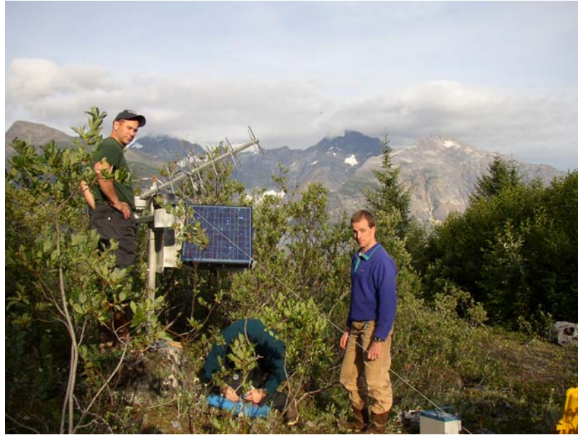
Figure 3. GOES site in Queen Inlet. GOES satellite transmission system transmits hourly data on precipitation and air temperature, while storing all data on a Campbell data logger located within the grey box. We are currently working on new systems to replace this unit and that at the Johns Hopkins which was completely destroyed by avalanches.
