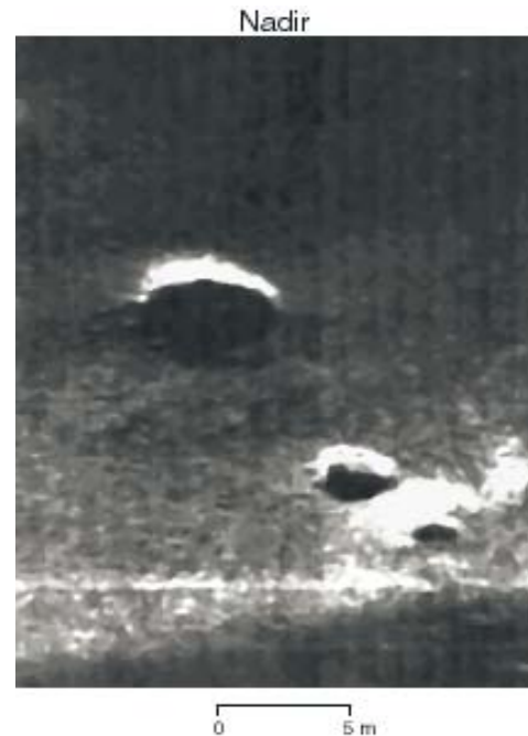
Figure 2.22b. Enlarged view of pits in Fig. 2.22a. Black and white have been reversed on image to give a somewhat different perspective of these pits. On this image white is high backscatter off black wall of pit, black is low backscatter from the hole or depression of the pit.
