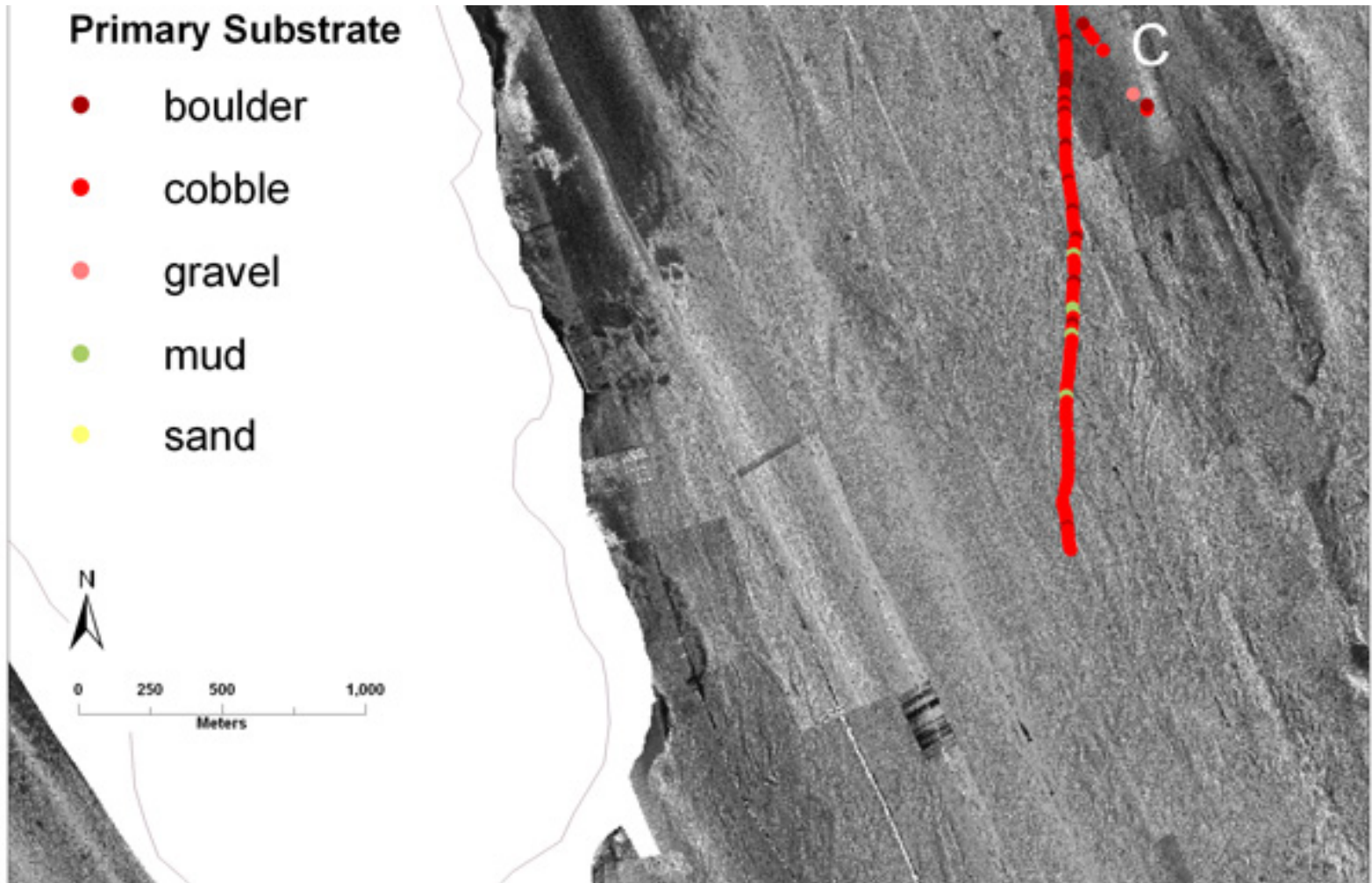
Figure 4. Acoustic backscatter data and video observations illustrate a region of transition in seafloor properties east of Willoughby Island, from soft, muddy sediment in the north (top) to coarse-grained boulders and cobbles in the south.
