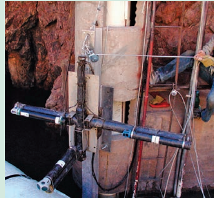
Three-frequency array of sideways-looking acoustic-Doppler current profilers deployed at the Grand Canyon streamgage
