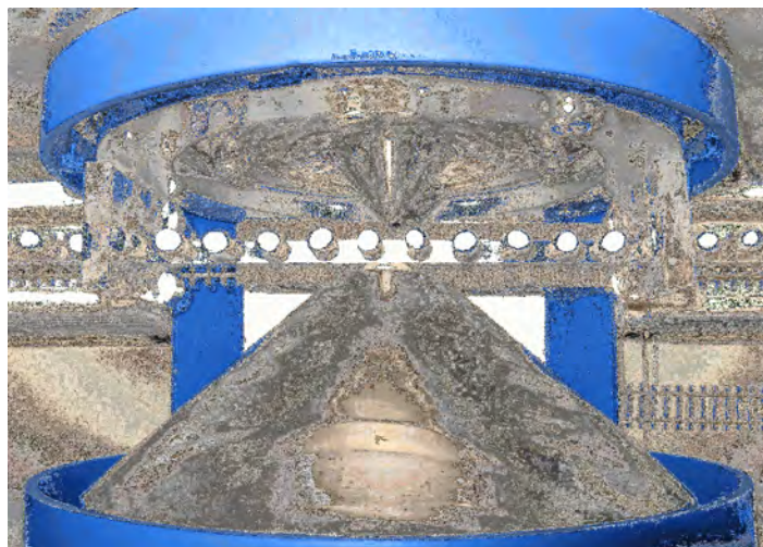
Figure 3. Ionization region of the DART through which an aluminum bar supporting cotton swabs is pulled. Two alignment devices determine the position of the swabs within the ionizing beam.
