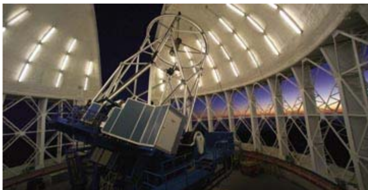
This image shows the Gemini North Telescope on the evening of April 19th, 2005 during evening twilight. Featured on the foreground of the telescope is the laser guide star (LGS) clean-room (blue box with white door). The Gemini solid-state sodium laser is located in this box and shines up through a network of tubes and relay optics (also visible) where the beam is "launched" by optics located behind the secondary mirror. Credit: Gemini Observatory
