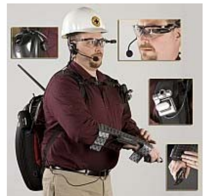
A demonstration of the EvacPack, a high-tech tool developed by the RESCUE team. The pack allows the user to send and receive up-to-the-minute information during a disaster response, including video, audio and text-based data. Credit: University of California, Irvine.
