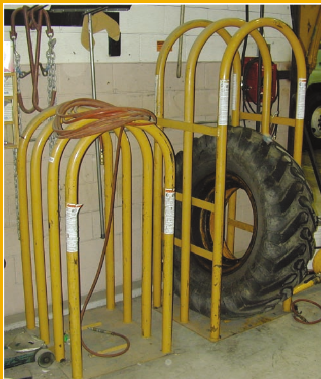
Replacing a damaged safety cage protected a worker when a tire he was inflating exploded.
