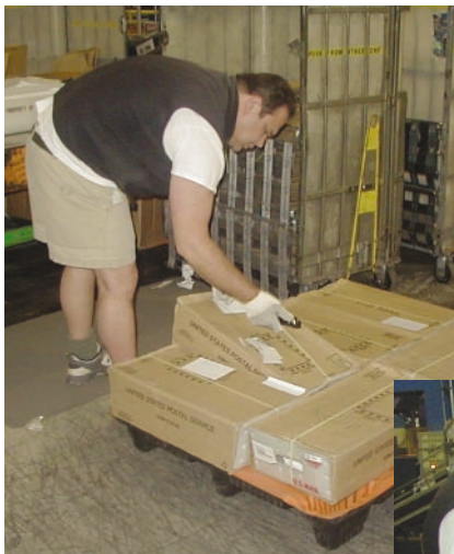
By elevating trays of letter mail for mail handler Steve Micare, right, the Albany Processing and Distribution Center eliminated the need for him to bend down and risk back strain, above.
