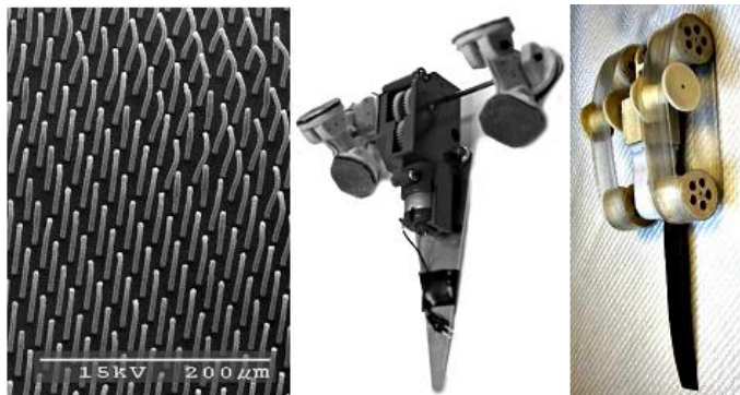
The left image shows an array of synthetic adhesive fibers 4mm in diameter that will be used to enhance the performance and robustness of climbing robots such as the ones shown in the center and right images climbing walls. Credit: Carnegie Mellon University
