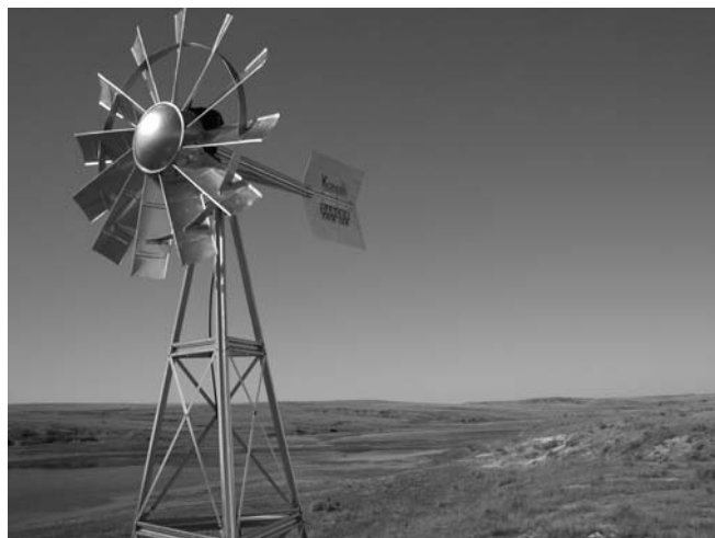
BLM-administered Homestead Reservoir sports a new aeration windmill installed to improve fish habitat, complete with a livestock-proof fence.
