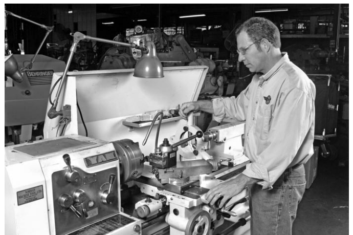
Tool and die makers use manual lathes to make custom parts or small batches of parts.
