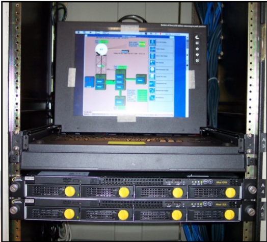
Part of the Radar Product Generator
