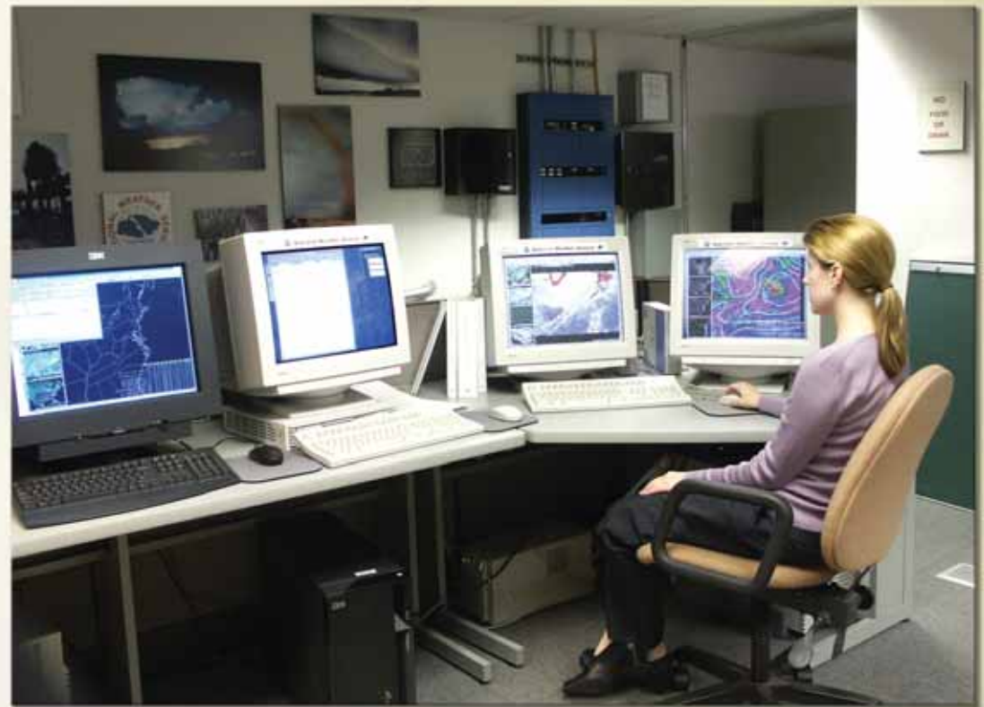
Through Advanced Weather Interactive Processing System (AWIPS) workstations, forecasters interact with a common digital database and use interactive forecast preparation tools to quickly and accurately prepare watches, warnings, and forecasts for dissemination.
