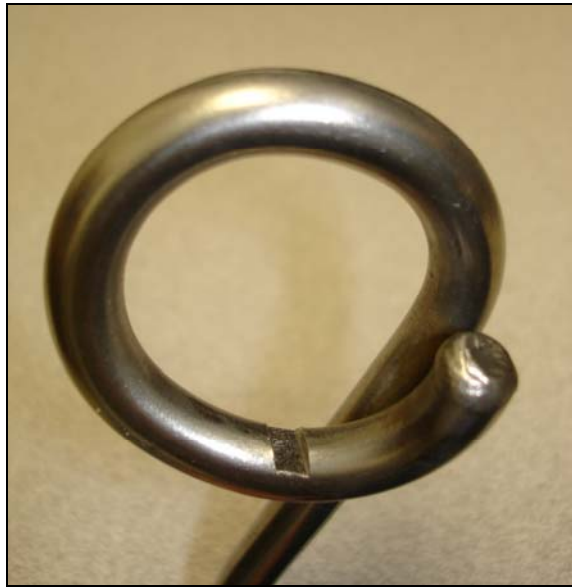
Figure 2-7 a, b and c. Notch the pigtail curl where the shank of the hook contacts the vertical bottom of the pigtail curl, ~1/16" - 1/8" deep and ~1/8" wide using a metal file [(a) Photo courtesy of ARC; (b) and (c) NMFS/SEFSC photos].
