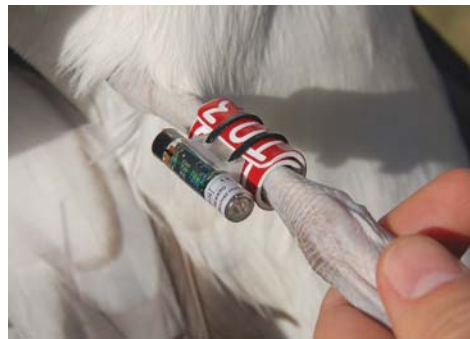
This light-weight geo-location device enables sea bird biologists to track long-range movements of tagged birds for up to two years.
