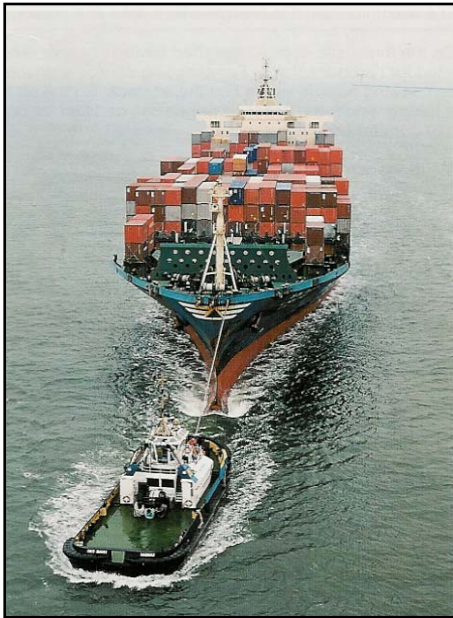
Figure 2-11. Tug towing Post Panamax container vessel from its bow.
