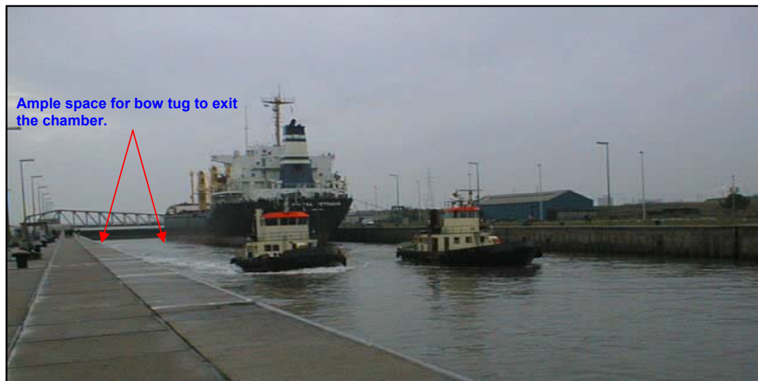
Figure 2-7. Bow tug exiting the chamber after docking maneuver is complete.
