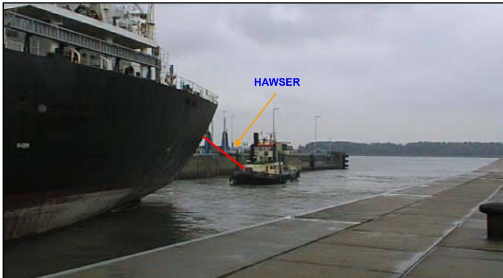
Figure 2-6. Stern tug using hawser line through center chock.
