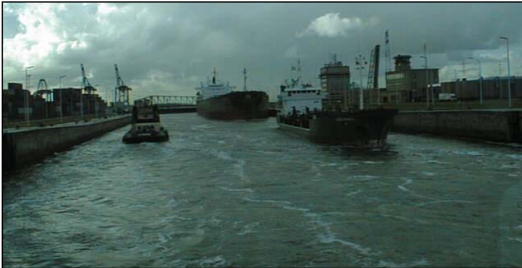
Figure 2-8. Tug entering chamber to assist vessel during the exiting maneuver.
