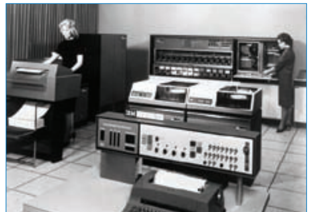
An IBM 1440 Data Processing System circa 1965. The 1440 was a low-cost system designed to solve the increasing data handling problems of smaller volume businesses, meeting the need for a complete accounting system and offering the benefits of a business information system. (Photo courtesy of IBM)
