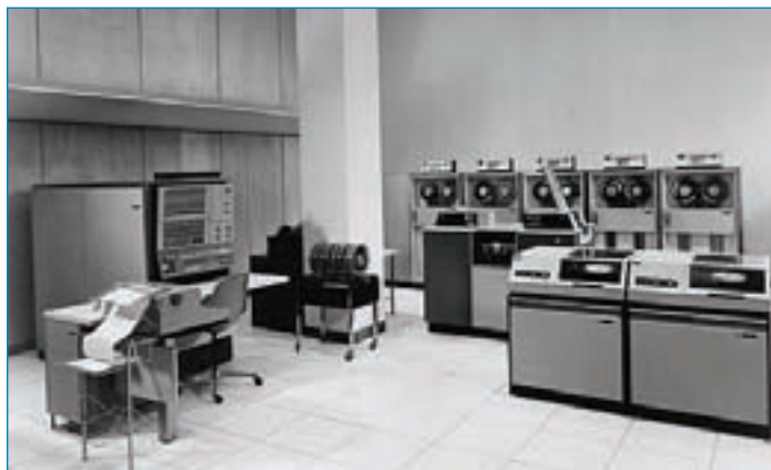
An IBM 360 Model 30 circa 1968. The smallest of the System/360 configurations, the Model 30 could serve as a stand-alone system, a communications system or the satellite processor of a larger system. (Photo courtesy of IBM)
