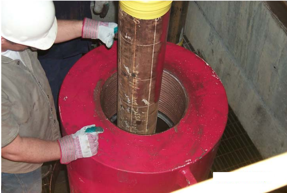
FIGURE 6-3 Typical Collapse Sample Being Installed Into Chamber
