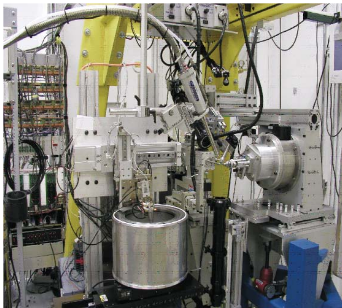
Fig. 1. The SER-CAT automounter installed on 22-BM.
