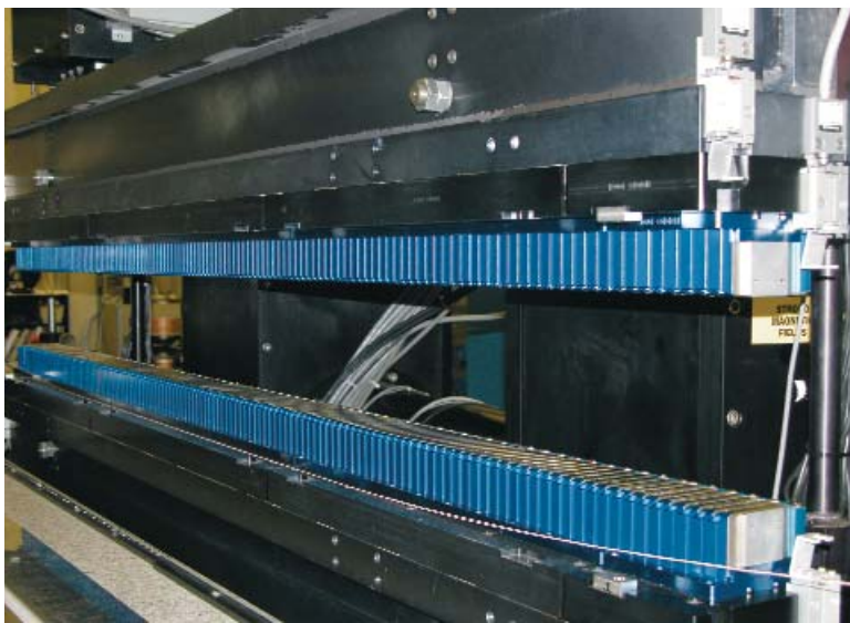
Fig. 1. The new SmCo undulator (3.5-cm-period length) in the magnet measurement laboratory prior to installation. The blue color is from anodizing of the clamps and not from the SmCo magnets. (Photo: Kurt Boerste [ASD])
