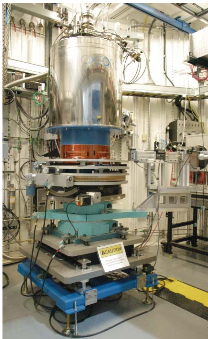
Fig. 1. The 13-T vertical-field cryogenic magnet shown mounted on a diffractometer. A polarization analyzer is mounted after two sets of slits on the 2\theta arm. A two-dimensional image plate is placed downstream to quickly collect diffraction patterns.
