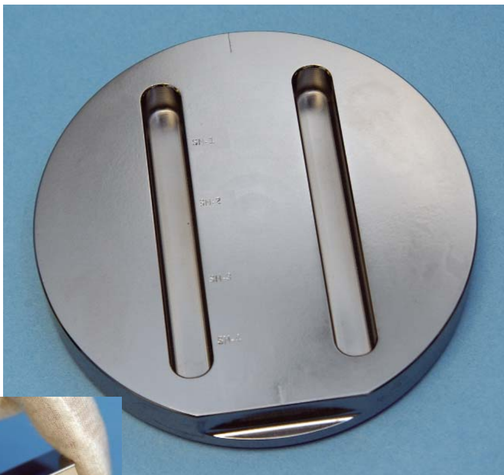
Fig. 1. Four state-of-the-art, elliptically shaped mirrors were produced from one parent substrate (top photo). The backside of the parent is shown here. After figuring the mirror front surface, the area between the channels is cut from the parent, and it is further cut perpendicular to the channel length to produce the four mirrors. Inset: The 40-mm-long palladium-coated mirror tested at the APS is shown. This is one of the four identical mirrors cut from the parent shown.
