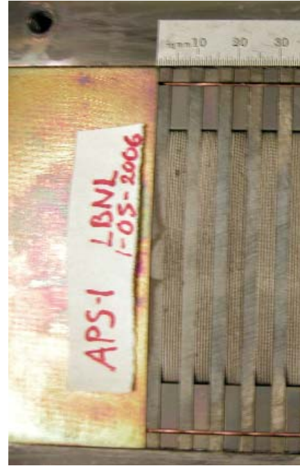
Fig. 5. A test section of undulator, designed, wound, and heat treated at LBNL. Another section is being prepared using ceramic-insulated wire. The LBNL design includes endshoes, at the top and bottom in the photo above, that provide additional support to the coil and help fill in voids.
